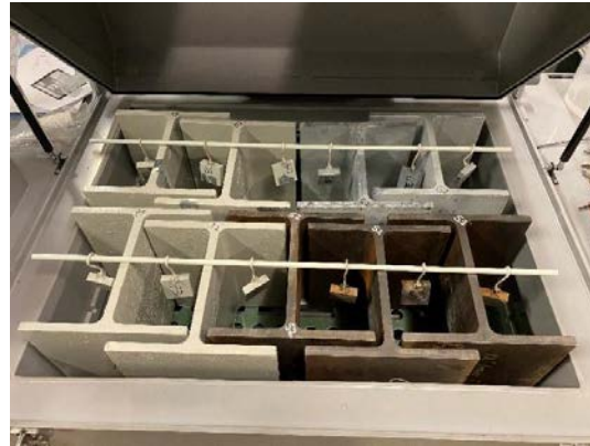
Figure 4. Samples inside the cyclic corrosion chamber
