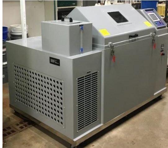
Figure 2. Cyclic corrosion test chamber
